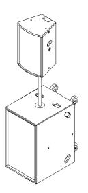
A top hat stand type fitting is mounted in the base of the cabinet for use with 35mm diameter loudspeaker stands with a load rating of at least 37kgs (82lbs).
